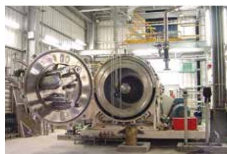
FIG. 2. Rousselet-Robatel horizontal peeler centrifuge with screw conveyor discharge.
